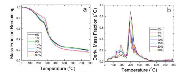
*Note*. Weight fraction of zein-citrate films up to 800 °C. Samples retain a higher mass overall but degrade much earlier than nanofibers. (b) First derivative of the remaining mass. The large presence of noise indicates thermal instability.
