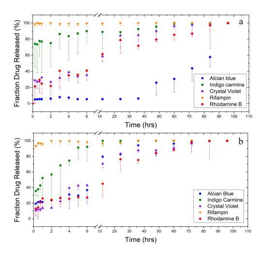
*Note*. Normalized release profiles of various model drugs from silk (a) fibers and (b) thin films. Error bars represent standard deviation.
