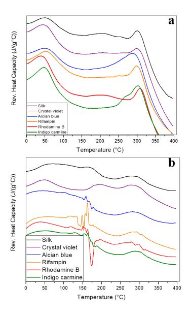
*Note*. Reversing heat capacity of silk and silk-model drug (a) fibers and (b) thin films. Exothermic is upward.
