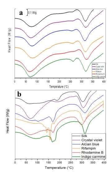
*Note*. Total heat flow graphs of silk and silk-model drug (a) fibers and (b) thin films. Exothermic is upward.
