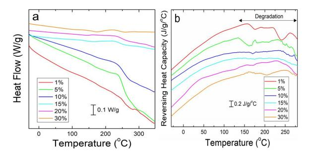
*Note*. (a) Heat flow thermogram of zein-citrate composite films. Degradation begins earlier than in nanofiber composites. (b) Reversing heat capacity thermogram shows noise due to the thermal instability of the composites beginning at 150 °C.
