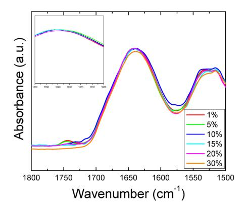
*Note.* Absorbance in the Amide I region in all zein fiber samples reverts to the 1640 cm<sup>-1</sup> seen in zein fibers without citrate. This indicates a reversible transition back to the original random coil structure of zein before citrate was embedded.
