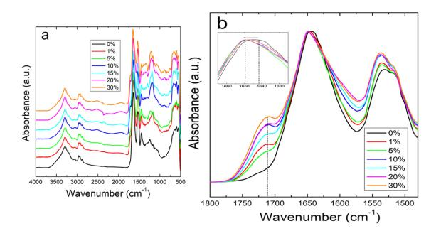
*Note*. (a) Full FTIR spectra. (b) Amide I and II Regions of Fibers. Unloaded fibers show a peak at 1640 cm<sup>-1</sup> indicative of random helical structure while fibers loaded with
