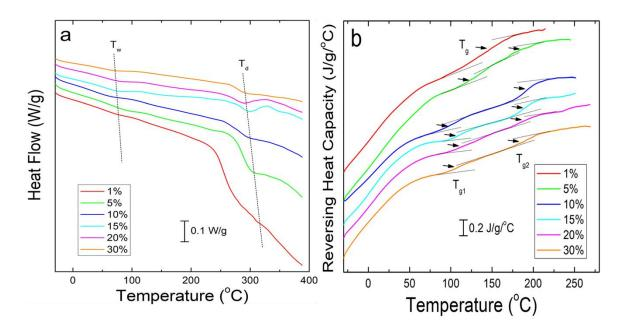
Note. (a) Heat flow changes at  $T_w$  due to water evaporation and  $T_d$  due to thermal degradation. (b) Step changes in reversing heat capacity can be found at  $T_{g1}$  and  $T_{g2}$  for the fiber samples with the drug. The step at  $T_{g1}$  is much more defined at higher wt% of citrate.
