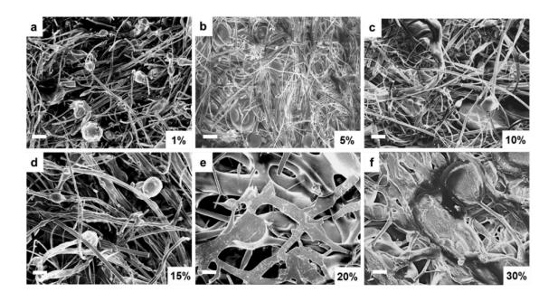
Note. Sodium citrate varies from 1 to 30 wt% citrate/zein: (a) 1 wt%, (b) 5 wt%, (c) 10 wt%, (d) 15 wt%, (e) 20 wt%, and (f) 30 wt% sodium citrate embedded nanofibers. (scale bar size: 10 μm).
