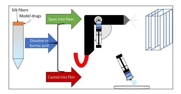
*Note*. Silk-model drug solutions were spun into nanofibers via spray gun or casted onto PDMS molds for film fabrication.
