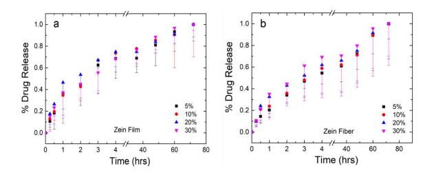
*Note*. Normalized release profiles of sodium citrate from corn zein films (a) and fibers (b). Content of sodium citrate ranged 5 to 30 wt% drug/zein with samples taken between 0.25–72 h.
