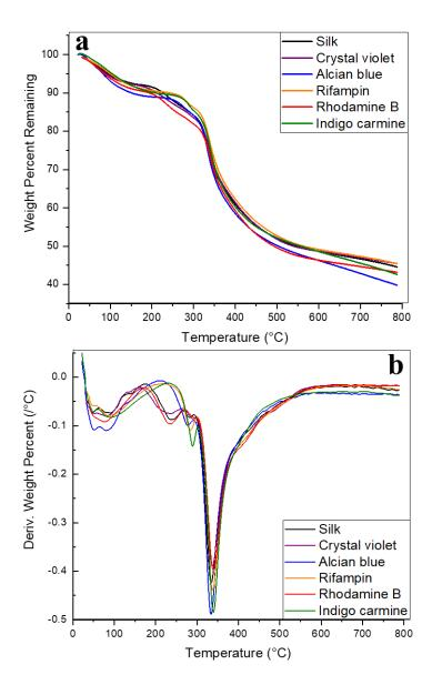
*Note.* (a) Remaining weight percent of silk and silk-model drug fibers as they were heated to 800 °C. (b) Derivative of remaining weight percentage curves.
