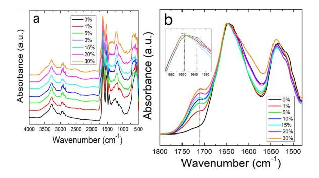
*Note*. (a) Full FTIR spectra. (b) Amide I and II regions for films. Unlike the nanofibers, there is an insignificant shift in absorbance peak when sodium citrate drug is embedded. Like in the fibers, all samples with citrate show shoulder at 1720 cm<sup>-1</sup> that scales with wt% of citrate.
