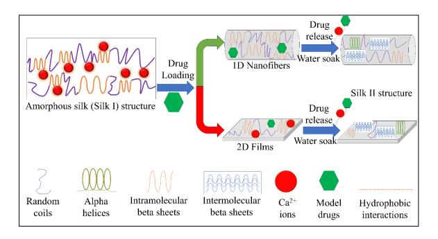
*Note*. Porous 1D fiber networks allow for the integration of model drugs, which then influence the self-folding behavior of silk protein. In flat 2D films, model drugs are unable to interact in the same way. As a result, fibers are able to protect embedded model drugs from thermal degradation and slow the release of the molecules from its structure. In thin films, the drugs are more susceptible to thermal degradation and there is less control over their release.
