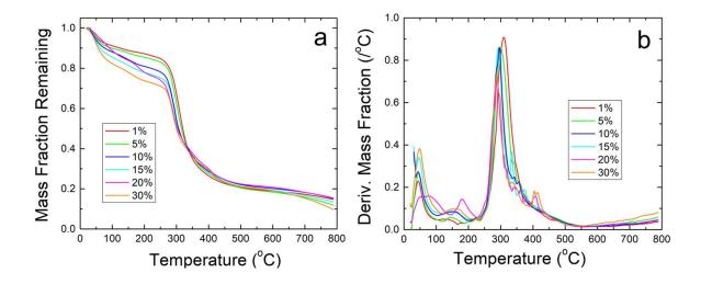
*Note*. (a) Weight fraction of zein-citrate nanofibers up to 800 °C. (b) First derivative of the remaining mass helps visualize two peaks due to bound water evaporation and zein degradation.
