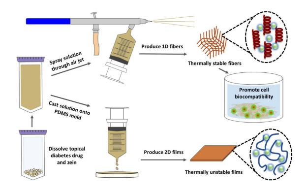
*Note*. Sodium citrate is embedded into 1D zein fibers or 2D zein films. 1D zein fibers have higher thermal stability and promote cell biocompatibility.
